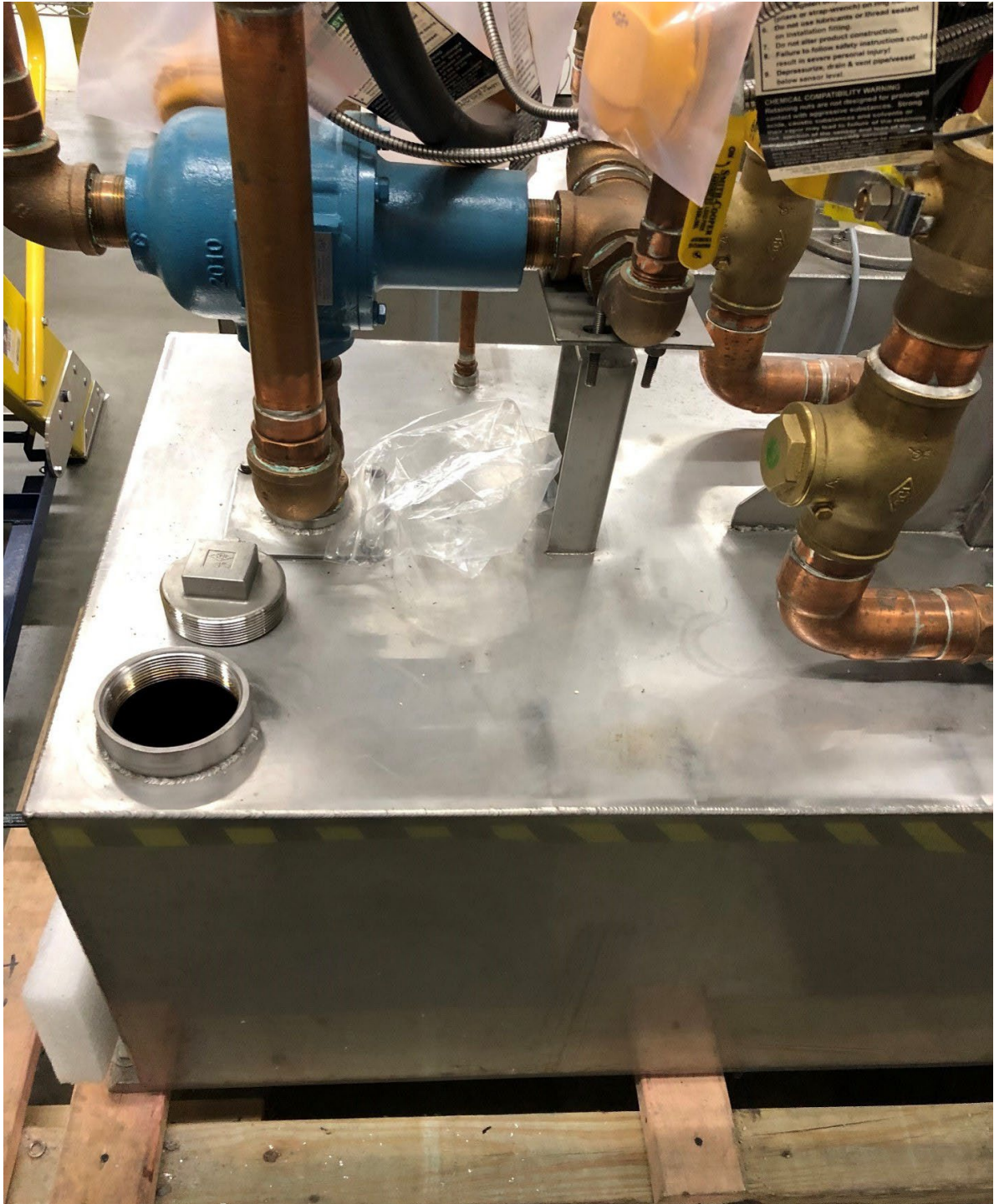
The coolant level should be between 3.0” to 3.5” from the top of the steel tank.
