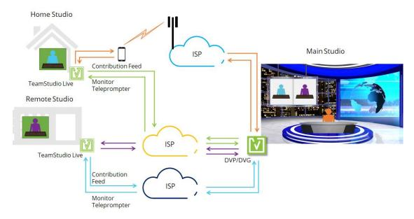
Secure in-band management via the VPN tunnel enables technicians at the main studio to remotely configure, troubleshoot, and manage VideoFlow devices as well as any other connected equipment at the remote studio.
