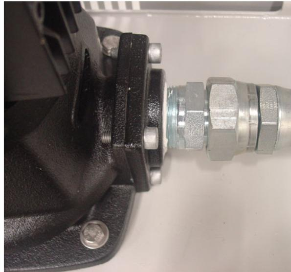
Male/flange nipple into the oil pump assy.
