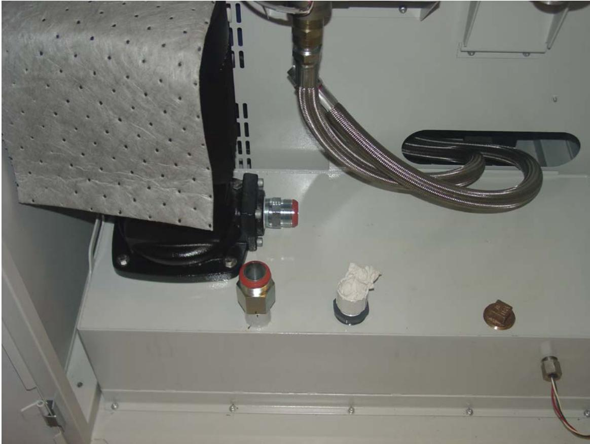
Red Flair-tite seals on tank return and pump flange tapered male ends
