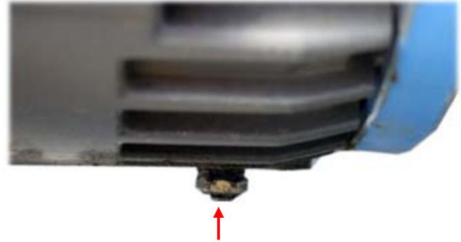
4. Clean grease fittings. Remove both grease outlet plugs on the bottom side of motor (opposite of each grease fitting) and place them in a clean safe place.
