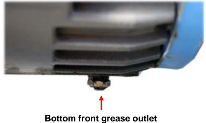
4. Clean grease fittings. Remove both grease outlet plugs on the bottom side of motor (opposite of each grease fitting) and place them in a clean safe place.
