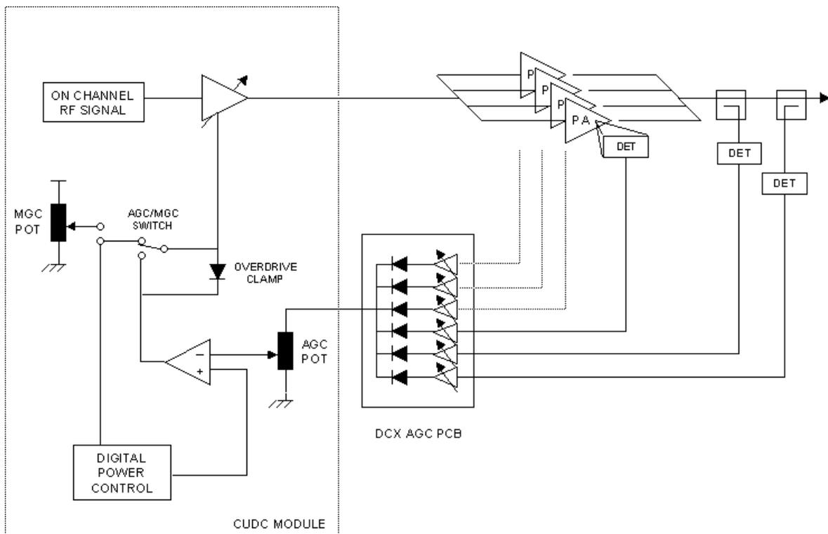
Figure 1. Simplified block diagram of transmitter gain control system.
