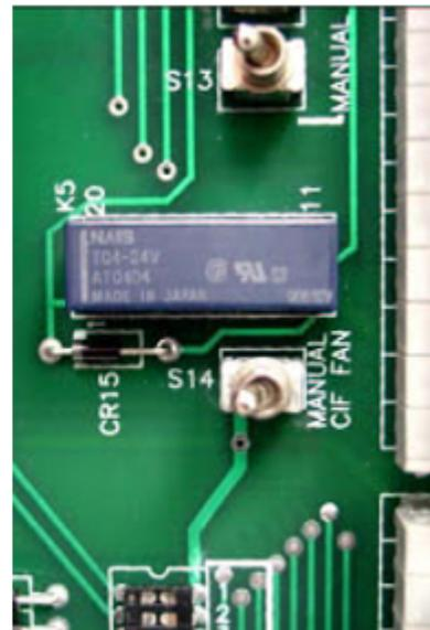
Manual C/F fan toggle switch S14 in off position
