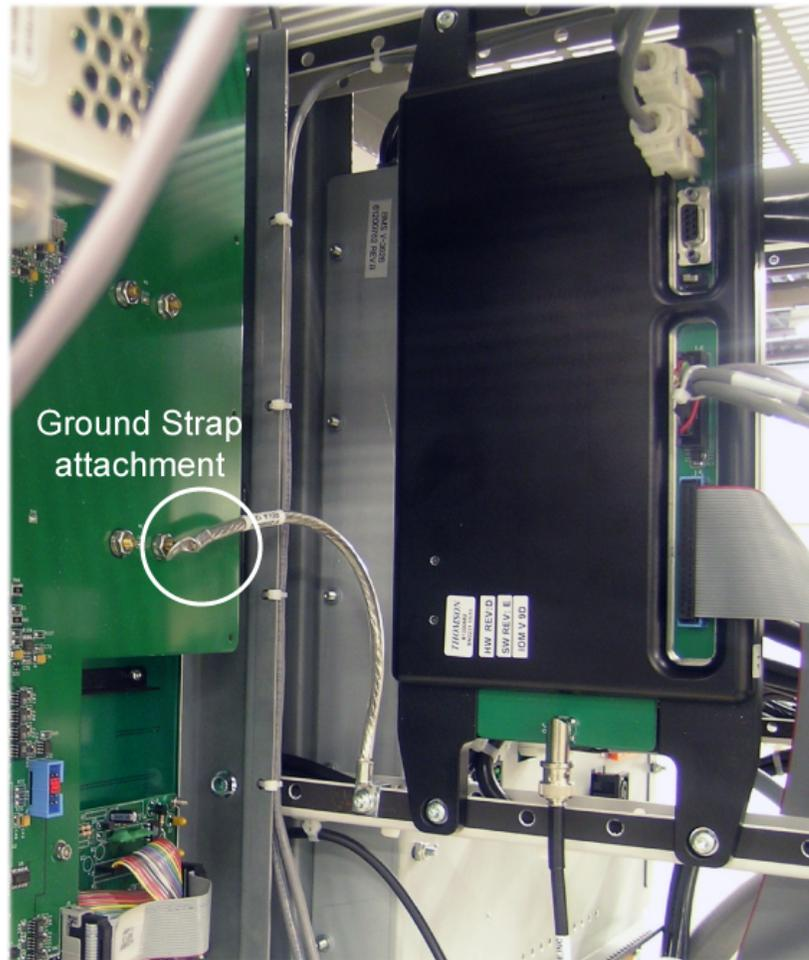
Install new speed nut and front panel ground strap
