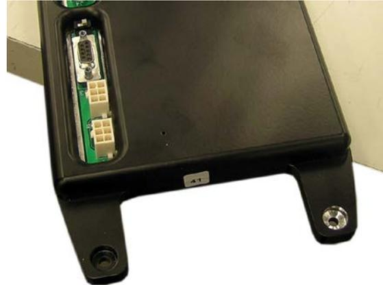
Paint removed from mounting hole
