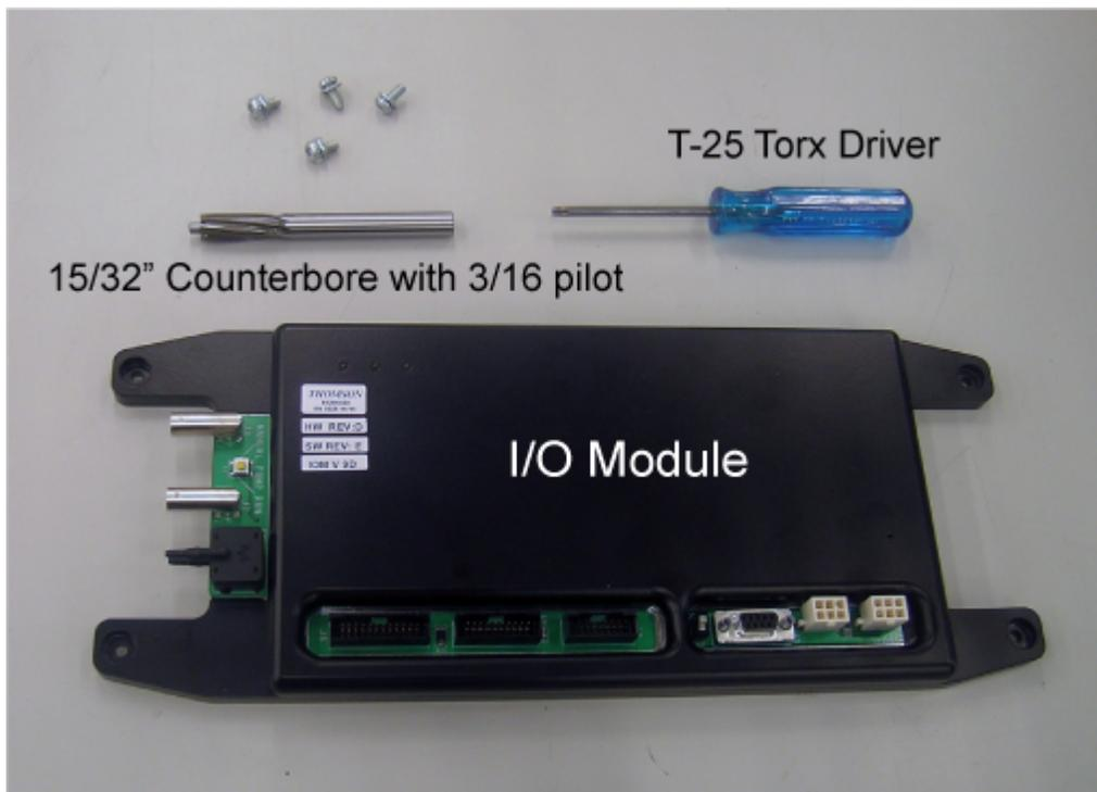
7. Insert the counterbore bit into the drill and hold the I/O module on a secure surface and slowly but carefully drill out the top left and bottom right mounting holes -- just enough to remove the paint. Avoid removing excessive amounts of metal during this process. Also keep any metal shavings generated during this process from getting into the module.
