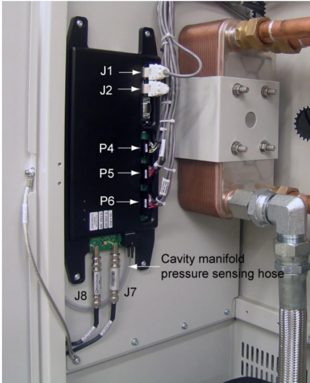
6. Use the T-25 Torx ® driver to remove the four screws from the I/O Module.
