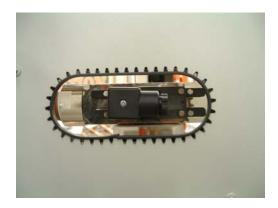
3. The trip pint is set by unlocking the armature/switch on the flow meter by loosening the two locking screws and sliding it along the length of the meter. There is a calibrated gauge on the side of the meter along with a corresponding mark on the switch. Where this mark lines up along the gauge scale determines the trip level of the switch. Once this is set per the correct value as seen on the gauge, tighten the two locking screws to hold the switch in position. See the pictures below.
