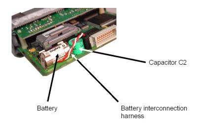
6. Remove 3V battery and interconnect harness from CPU module.
