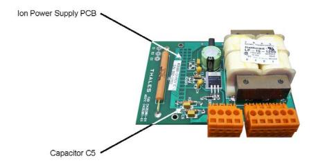
A .01uF ceramic disk capacitor may be obtained free-of-charge by contacting Comark Customer Service at 1-800-345-9295 (request part number 700262-01) or purchased at a local electronics supply store (Radio Shack #272-131 .01uF 500WVDC or equivalent)
