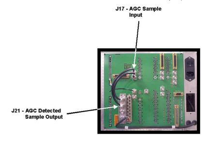
**NOTE:** The AGC circuit requires at least +2V DC of rectified output sample at J17 to function properly. This level may be achieved by relocating all RF attenuator pads to the final exciter output at J23. This makes the final amplifier work harder, thereby increasing its detected output sample at J21.
