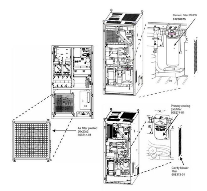
This service bulletin contains two procedures addressing periodic maintenance of the cooling system in the DCX Paragon HPA cabinet. More specifically, procedures are provided for the periodic replacement of the air filter elements and the primary cooling loop oil filter, for those HPA cabinets with an oil-cooled IOT. The assemblies discussed in this bulletin are identified in the illustration above.
