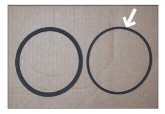
7. Moisten new gasket with oil and carefully install it in groove where old gasket was previously located.
