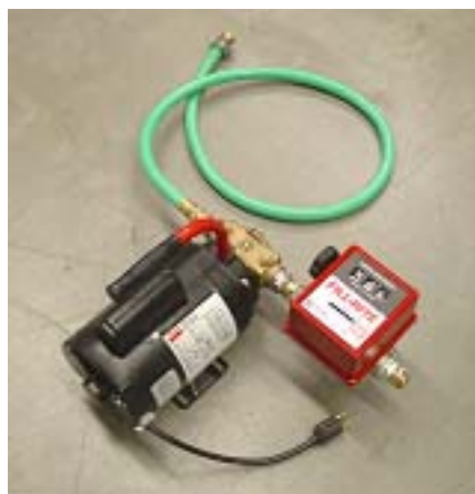
Pump & gauge assembly.
