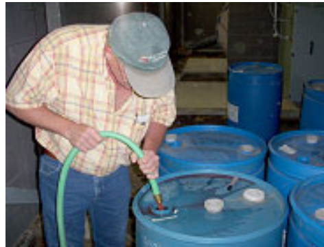
Pump used solution into waste barrels
