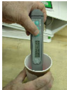
Test solution % with refractometer
