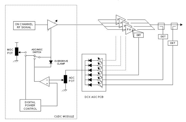
Figure 1. Simplified block diagram of transmitter gain control system.
