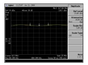
**NOTE:** Markers in this series of photographs are at +/- 4MHz from channel center. That is, they show an 8 MHz wide frequency band.
