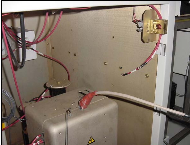
Photo of high pot test set HV- lead to FBI supply body.
