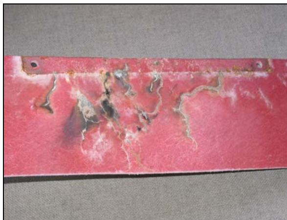
Figure 1. Photograph of HVPS resistor board showing deterioration.
