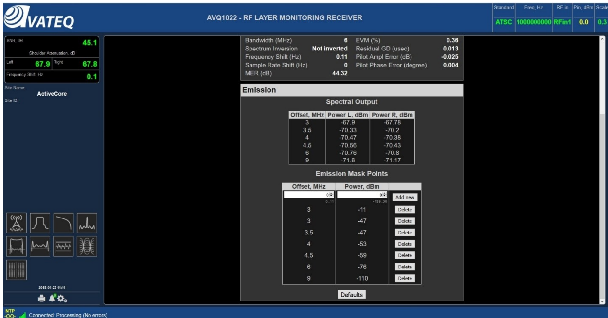
Figure 7. Pre-set Emission Mask and Spectral Output
