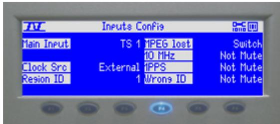
The second page under F4 menu allows input configurations of the main MPEG input and clock sources. It also defines what actions will be taken in the event that one of these parameters falls outside the normal operating state.
