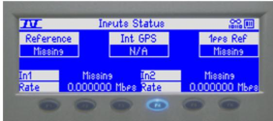
The first page under the F4 function key depicts the input status of the exciter. These signals include the timing references and the transport stream inputs. The Inputs Status screen displays the following parameters:
