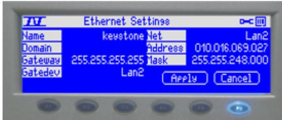
The fourth time the F6 button is pressed will yield the Ethernet settings page. Note the exciter must be rebooted if any network setting is changed. The change will not take effect until the unit has rebooted.
