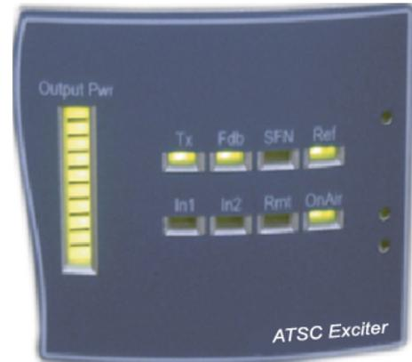
**Tx:** - Indicator will be green when the transmitter is commanded to enter the transmit mode. This is different than the actual on-air status, and indicates the desire for the transmitter to go on-air. For example, there may be a condition where the transmitter is placed in transmit mode but an out of tolerance condition prevents the on-air status.
