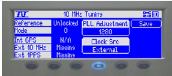
When F4 is pressed a third time the menu for 10MHz tuning is displayed. This menu displays status regarding the onboard reference source / PLL system. PLL adjustment is mostly used when both internal and external clock sources are missing, and the modulator is defaulted back to the internal OCXO.
