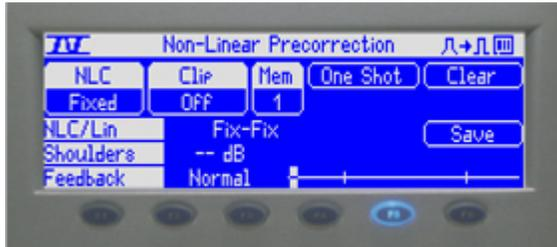
The first menu within F5 function key is Non-Linear Precorrection. This allows compensation of the non-linear distortions that occur when maximizing the output power and efficiency of the power amplifier stages. This compensation is performed digitally by processing a feedback sample taken from the transmitter output, which has been down-converted and brought IF for digital signal processing.
