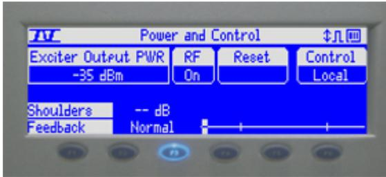
The F3 menu is the first menu that has user controls; the first press of the F3 button displays the Power and Control page. The following controls are available:
