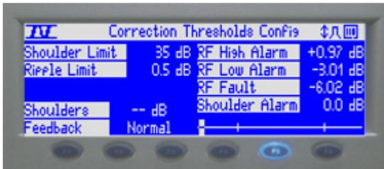
This menu is displayed when the F5 button is pressed three times. It allows threshold configuration of various RF alarms.
