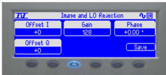
If the F3 function key is pressed a third time, the image and LO rejection control page is displayed. These controls are used to null the LO and image frequencies, the undesired products of the mixer stage. These are the results of the first upconversion stage within the transmitter used to convert the 27.5MHz IF to the UHF channel. A detailed procedure to accomplish the proper alignment of these parameters is outlined in the *ADAPT IV Installation Manual*.
