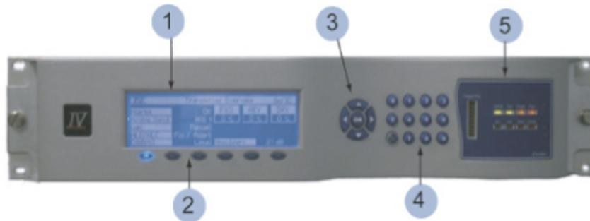
1. LCD display: - The Liquid crystal display is a part of the Man-Machine-Interface (MMI) for local control and monitoring of the transmitter RF performance. Selecting function keys F1 through F6 can change the displayed menu. A screen saver and display intensity function is available. Press and hold the menu/shift button then select F1 to toggle to screen-saver mode, or press F3 to adjust display intensity.
