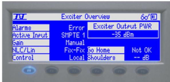
The first page under the **F1** menu displays the transmitter overview. This screen provides the current status and mode for which the transmitter is operating. This is a status-only screen and no user adjustments are available. The transmitter overview screen functions are as follows:
